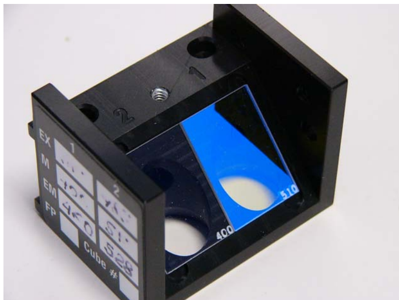
Figure 2: Mirrors positioned in the filter cube
