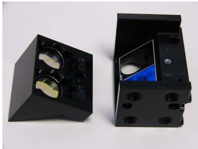
Figure 5: Filter cube with top removed
