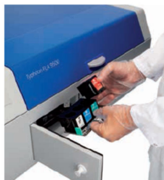
Fig 2. Filters are easily exchanged by the user.
